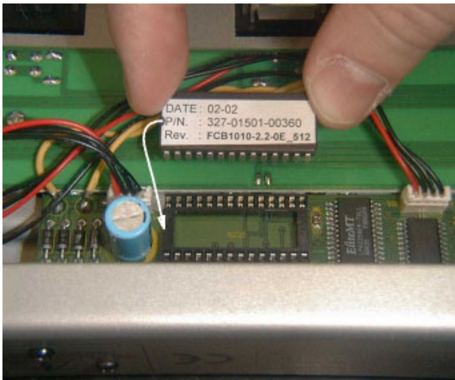
Fig. 1.2: Exchanging the EPROM
