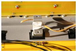
Now take the 2 stripped wires of the cable unit which connects MIDI connector board and main electronics board, and connect them to the 2 pieces of yellow wire you left on the main electronics board. In case you have a soldering iron, you can directly solder the 2 black wires to the electronics board instead. It is NOT important which wire is connected to which terminal, a rectifier circuit will always create the correct polarity on the main board.
