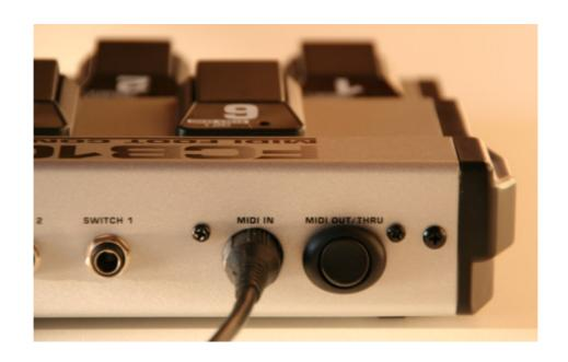
Last thing to test is the 2-way communication. Connect the short red MIDI cable from converter box MIDI OUT to controlled device MIDI IN, and the blue MIDI cable from controlled device MIDI OUT to converter box MIDI IN. Now check that everything works exactly as before the upgrade, only without the cable mess at the floorboard side... Congrats!
