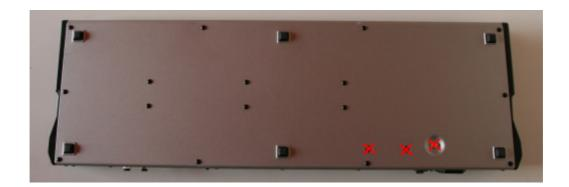
Attention: a ground lead attaches the bottom plate to the FCB1010 chassis. It is not necessary to remove this connection, just lay down the bottom plate close to the chassis while doing the upgrade.
