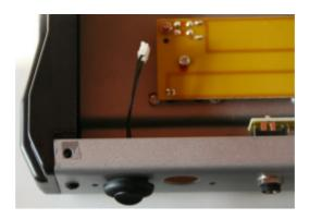
Now install the new connector board, using the same 2 screws which held the original board. While doing so, push the dangling power switch cable up, so it will be close to the matching jack on the connector board. After installing the connector board you can plug in the power switch cable, as shown below.
