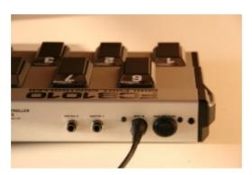
At the other side of the MIDI cable, a small standalone box converts the combined 7-pin connector back into 3 separate connectors: PWR IN, MIDI IN, MIDI OUT. You can use any regular 9V DC power adapter, delivering at least 500 mA, to phantom power your FCB1010.
