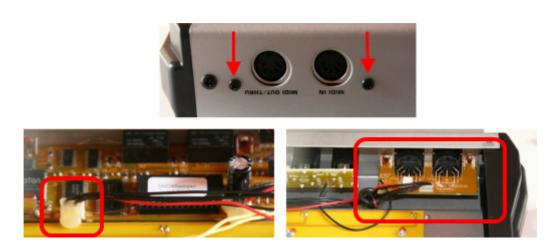
A small ground wire runs from MIDI connector board to jack board. You can just cut this wire close to the jack board.
